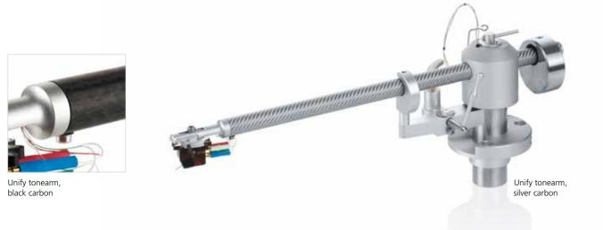
The Unify tonearm represents the summit of unipivot radial tonearms, and stands out not only for its elegant looks. A sapphire bearing and a hardened, precision polished steel tip are at the heart of a tonearm made of the best materials - and probably one of the best unipivot constructions in the high-end audio history. The base consists of a stainless steel pillar, the arm is made of carbon fibre and the bell is made of aluminium. This clever mix of materials guarantees resonance-free behaviour
